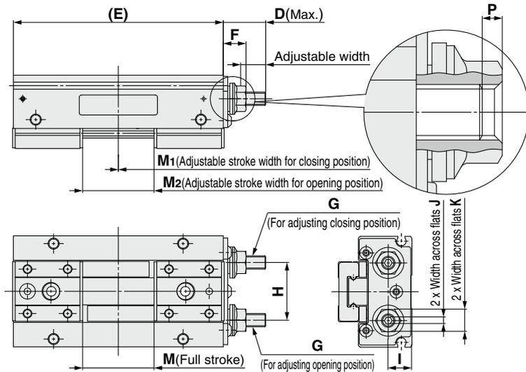
**Adjustable finger opening position type/MHF2-□-X83B1
