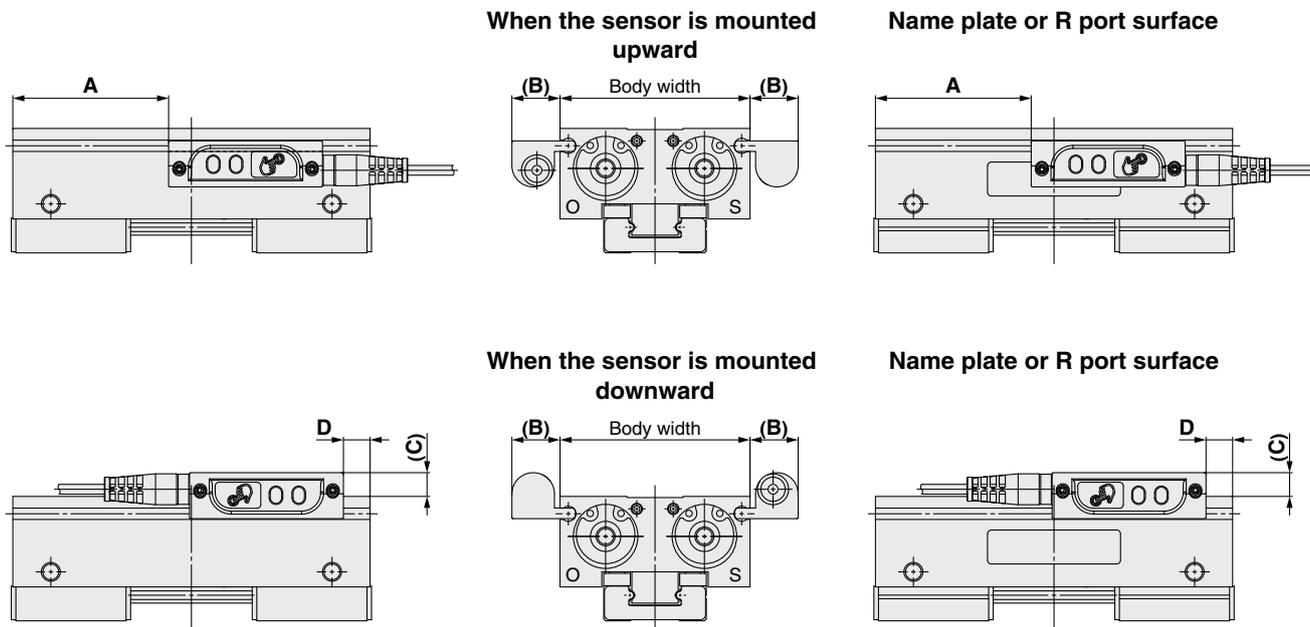
**Actuator Position Sensor Mounting Position Guide**
