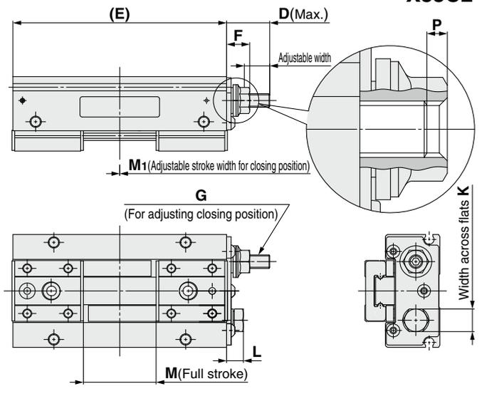
**Dimensions** (The □ in the table below indicates the symbol for stroke adjustable side (A: Adjustable finger opening/closing position type, B: Adjustable finger opening position type, or C: Adjustable finger closing position type).) [mm]
