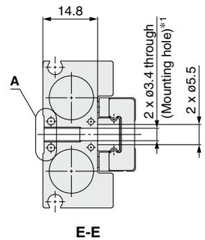
\*1 Use the attached hexagon socket head cap screws for mounting holes.
