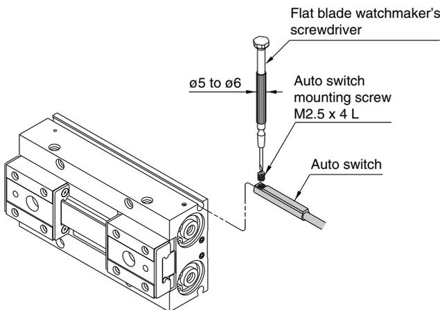
\* Use a watchmaker's screwdriver with a grip diameter of 5 to 6 mm to tighten the auto switch mounting screw. Also, tighten with a torque of about 0.05 to 0.15 N·m, or about 0.05 to 0.10 N·m for D-M9□A(V).
