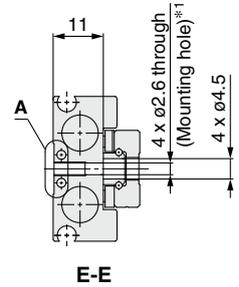
\*1 Use the attached hexagon socket head cap screws for mounting holes.
