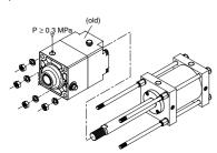
Similarly, apply 0.3 MPa or more of compressed air to the unlocking port of the new lock unit, and replace the new lock unit's temporary axis with the previous piston rod assembly.
