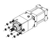
Apply compressed air of 0.3 MPa or more to the unlocking port, and remove the lock unit.
