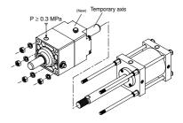
4) Tighten the tie-rod nuts (4 pcs.) on the rod side of the cylinder using a socket wrench.
