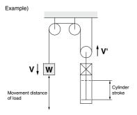
3. The following selection example and procedures are based on use at the intermediate stop (including emergency stops during the operation). However, when the cylinder is in the locked state, kinetic energy does not act upon it. Under these conditions, use the load mass at the maximum speed (V) of 100 mm/s shown in graphs 5 to 7 on page 955 depending on the operating pressure and select models.
