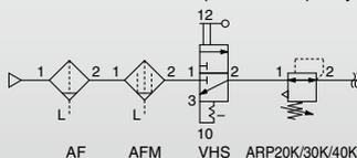
When the air supply is cut off and releasing the inlet pressure to the atmosphere, the residual pressure release of the outlet side can be ensured for a safety purpose.
