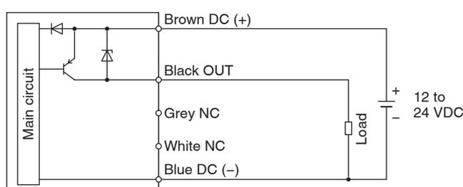
**When used as an IO-Link device**
