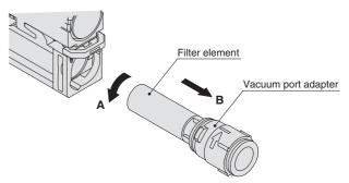
• When installing the filter, insert the filter to the end so that there is no gap or bending between the filter and the vacuum port adapter. The gap or bending will cause the element to deform inside the case.
