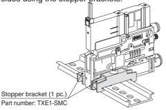
2. To mount a single unit onto the floor, use the optional bracket.
