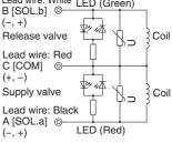
Light/surge voltage suppressor circuit is equipped for both single and double solenoid. Red LED turns on when supply valve (SOL.a) is energised. Green LED turns on when release valve (SOL.b) is energised.
