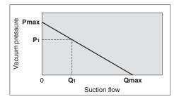
Flow rate characteristics are expressed in ejector vacuum pressure and suction flow. If suction flow changes, the vacuum pressure will also be changed. Normally this relationship is expressed in ejector standard operating pressure use. In graph, **Pmax** is maximum vacuum pressure and **Qmax** is maximum suction flow. The values are specified according to catalogue use. Changes in vacuum pressure are expressed in the below order.
