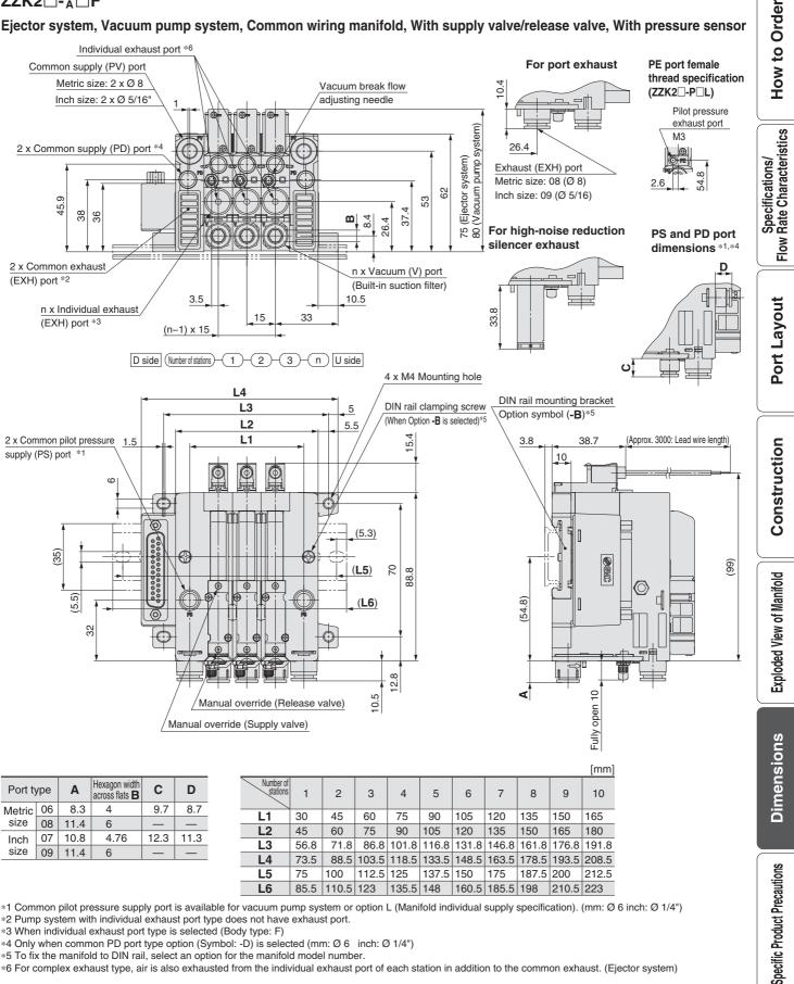
\*1 Common pilot pressure supply port is available for vacuum pump system or option L (Manifold individual supply specification). (mm: Ø 6 inch: Ø 1/4") \*2 Pump system with individual exhaust port type does not have exhaust port.
