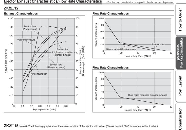
ZK2 15 Note 8) The following graphs show the characteristics of the ejector with valve. (Please contact SMC for models without valve.)
