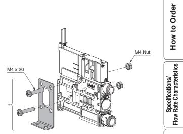
\*Mounting bracket for single unit (Option), [Nuts and bolts are included.] Part number: ZK2-BK1-A
