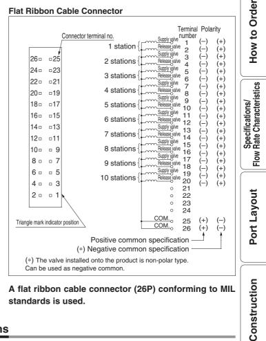
A flat ribbon cable connector (26P) conforming to MIL standards is used.
