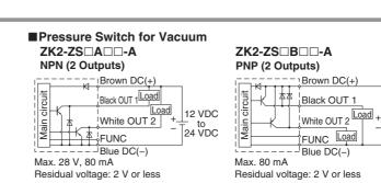
\*The FUNC terminal is connected when using the copy function. (Refer to the Operation Manual.)
