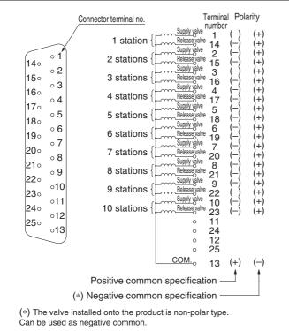
A D-sub connector (25P) conforming to MIL standards is used.
