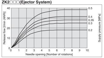
The actual suction flow at the point of suction varies depending on the piping conditions to the vacuum port. (The above graph shows the value of the ZK2B07.)
