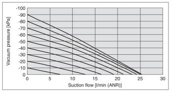
The actual suction flow at the point of suction varies depending on the piping conditions to the vacuum port. (The above graph shows the value when V port is Ø 8.)
