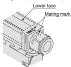
• If it is difficult to remove the vacuum port adapter, you can remove the adapter with a hexagon wrench using the hexagonal hole in V port. The table shows the port size and the width across flats.
