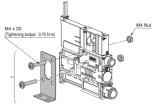
\*Mounting bracket for single unit (Option), [Nuts and bolts are included.] Part number: ZK2-BK1-A
