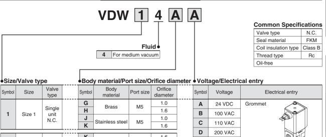
K 1.6 L 2.3 M5 M 3.2 Brass N 1.6 Р 1/8 2.3 O 3.2 Single 2 Size 2 unit R 1.6 N.C. S M5 2.3 Т 3.2 Stainless steel П 1.6 V 1/8 2.3 W 3.2 Ε 230 VAC Z Other voltages
