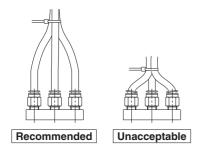
Fig. 2 Binding tubes with bands
