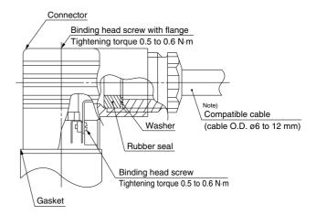
Note) For an outside cable diameter of ø9 to 12 mm, remove the internal parts of the rubber seal before using.
