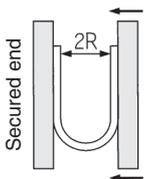
At a temperature of 20 °C, the tubing is bent into a U shape with one end fixed in position and the other end is gradually moved closer to the other end. The 2R measurement is made at the point where there is a 10 % change in the outer diameter of the tube.
