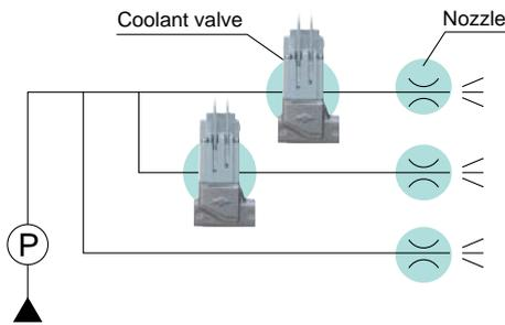
Pressure loss is improved by making the effective area ratio 2 : 1 between the upstream side and the nozzle.
