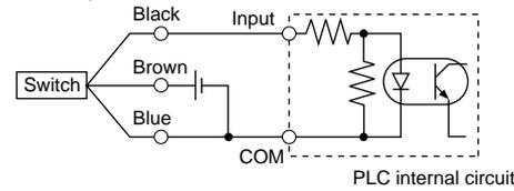
Connect according to the applicable PLC input specifications, since the connection method will vary depending on the PLC input specifications.
