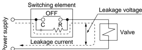
AC coil: 8% or less of rated voltage
