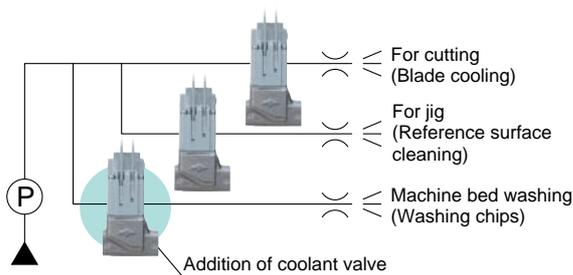
Stop machine bed-washing all the time. Machine bed washing can be stopped when coolant is flowing for cutting or jig by means of an additional valve.
