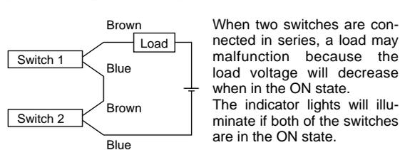
When two switches are connected in series, a load may malfunction because the load voltage will decrease when in the ON state. The indicator lights will illuminate if both of the switches are in the ON state.
