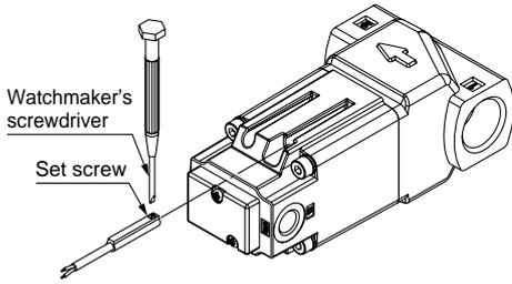
When tightening the auto switch mounting screw, use a watchmaker's screwdriver with a handle of approximately 5 to 6 mm in diameter. Furthermore, use a tightening torque of approximately 0.10 to 0.20 N·m.
