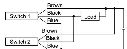
The indicator lights will illuminate when both switches are turned ON.
