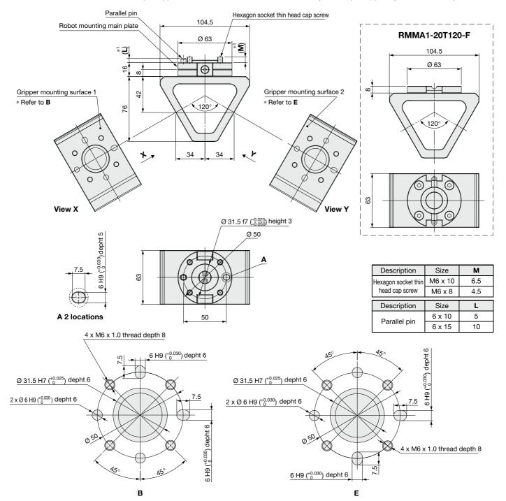
\*1 Two types of main plate mounting bolts and two types of parallel pins, with different lengths, are supplied with the product. Select parts that suit the robot in use.
