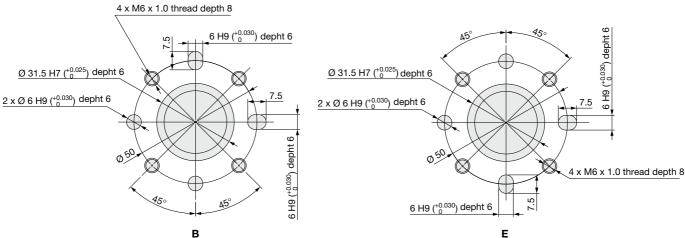
\*1 Two types of main plate mounting bolts and two types of parallel pins, with different lengths, are supplied with the product. Select parts that suit the robot in use.
