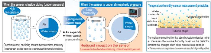
\* The atmospheric pressure relative humidity value displayed is lower than that of the relative humidity inside piping (under pressure). For the relative humidity conversion method, refer to "Set value (threshold value) setting" on page 3.
