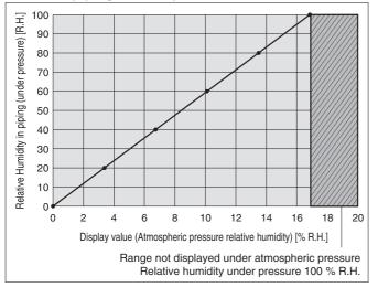
When the piping internal pressure is 0.7 MPa
