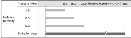
The range of atmospheric pressure and relative humidity that the condensation checker can measure changes depending on the pressure inside the piping (under pressure). For example, if the pressure inside the pipe (under pressure) is 0.3 MPa and the relative humidity is 100 % (maximum value), the atmospheric pressure relative humidity when released into the atmosphere will be 25.0 % R.H..
