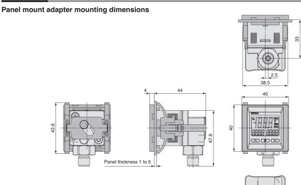
Panel mount adapter + front protection cover mounting dimensions
