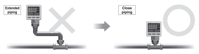
If the product is separated from the original piping, accurate measurements will no longer be possible due to external disturbances such as temperature variation in the extended piping. In addition, increasing the distance from the original piping slows down the temperature transmission and the response. Direct mounting to the piping is recommended.
