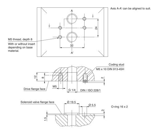
The solenoid valve can be attached with 2 mounting bolts.
