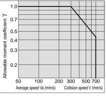
Note) Use the average speed when calculating static moment. Use the collision speed when calculating dynamic moment.
