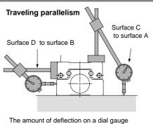
when the guide block travels a full stroke with the body secured on a reference base surface.
