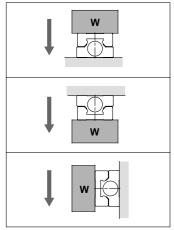
Note) No need to consider this load factor in the case of using perpendicularly in a vertical position.
