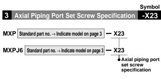
The axial piping port plug (M-3P, M-5P) is changed to a hexagon socket head set screw, and the overall length is shortened.
