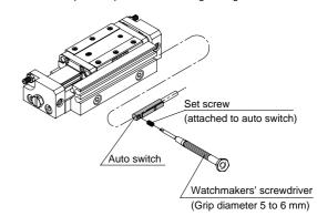
Other than the models listed in "How to Order", the I following auto switches are applicable. I For detailed specifications, refer to Best Pneumatics.
