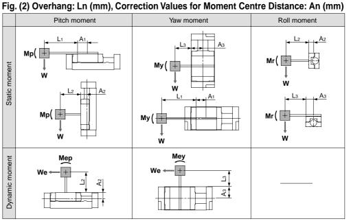
Note) Static moment: Moment by gravity Dynamic moment: Moment by stopper collision
