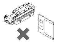
7. Do not attach magnets to the table (guide block) section.
