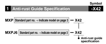
Martensitic stainless steel is used for the body, table and guide block, but if greater rust prevention is required use this specification.
