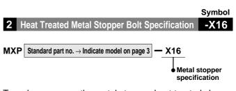
To reduce wear on the metal stopper, heat treated chrome molybdenum steel (SCM435) is used for the stroke adjustment screw.
