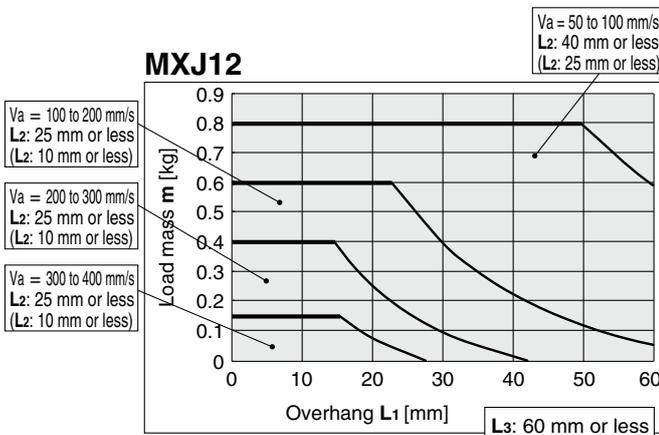
\* When the end plate is mounted, the value in brackets applies for  $L_2$ .
