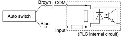
Connect according to the applicable PLC input specifications, as the connection method will vary depending on the PLC input specifications.
