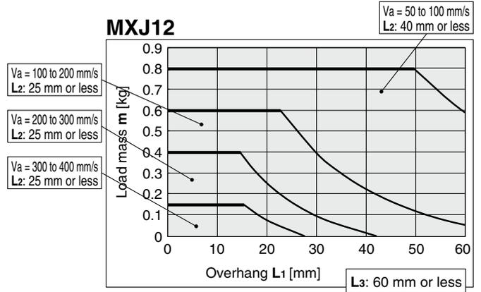
\* Confirm that the overhang  $L_1$  is within the allowable range based on the load mass and average speed.
