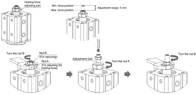
Turn the nut B to loosen while holding the nut A. (Nuts are tightened to a specified torque around the maximum holding force position (zero adjustment).) 2. Hold the adjustment bolt while holding the workpiece. Turn the nut A to adjust the holding force.
