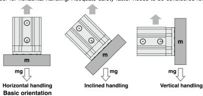
• Thin workpieces may be deformed during transportation. It is recommended to use multiple magnet grippers for scenarios such as this.
