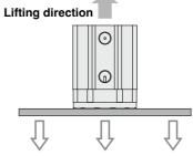
• Consider the centre of gravity of the workpiece to avoid moments being applied to the magnet gripper as much as possible.
