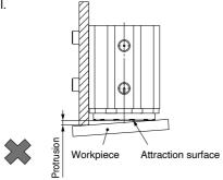
11. When multiple magnet grippers are used side by side, mount them so that the attraction surfaces are not uneven.
