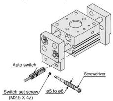
Note) Use a watchmakers screwdriver with a grip diameter of 5 to 6mm to tighten the auto switch set screw. Use a tightening torque of 0.05 to 0.1 Nm. As a rough guide, tighten the screw an additional 90° after feeling a tight resistance.
