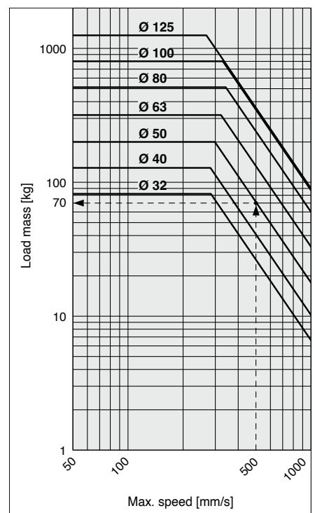
Example) Load limit at the rod end when an air cylinder with a bore size of Ø 50 is actuated at 500 mm/s. Extend upward from 500 mm/s on the horizontal axis of the graph to the intersection point with the line for a 50 mm bore size, and then extend leftward from this point to find the load of 70 kg.
