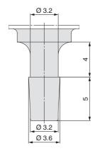
Recommended tubing diameter: I.D. Ø 2 to Ø 3.2, O.D. after mounting Ø 8 or less
