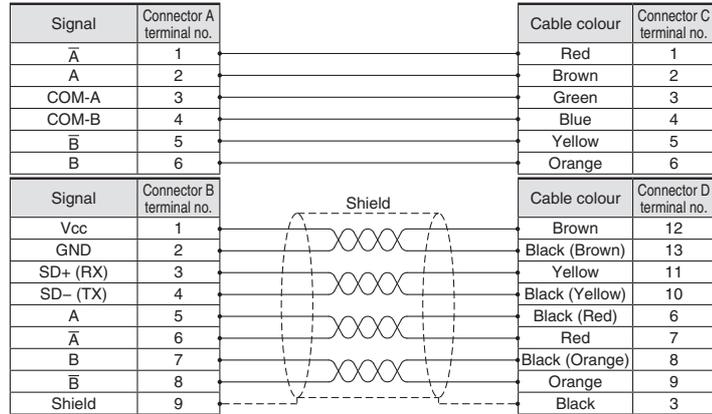
[Metal connector robotic cable with lock for battery-less absolute (Step motor 24 VDC)]
