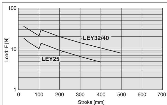
[Stroke] = [Product stroke] + [Distance from the rod end to the centre of gravity of the workpiece]
