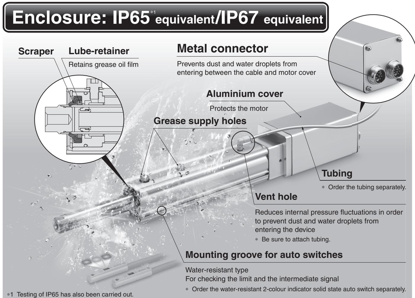
\*1 Testing of IP65 has also been carried out.
