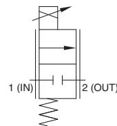
\* When the valve is opened, flow is blocked from port 1 to port 2. However, if the pressure in port 2 is higher than port 1, the valve will not be able to block the fluid and it will flow from port 2 to port 1.
