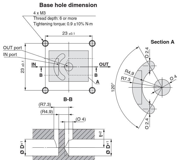
\*1 For  $\text{O } D$  dimension, we recommend  $\text{O } 8.2$  (equivalent to  $Rc 1/8$  pilot hole) or larger.
