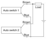
(Solid state) When two auto switches are connected in parallel, malfunction may occur because the load voltage will increase when in the OFF state.
