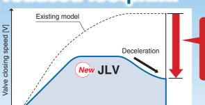
Impact energy when the valve is closed (Proportional to V<sup>2</sup>) **DOWN 90 %**
