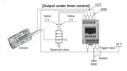
■Solenoid valves up to 24 VDC (4 W) etc. are controllable.
