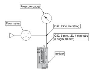
Fig. 1: Flow rate characteristics measuring circuit
