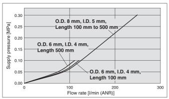
When a pressure above each line is used, the maintenance warning function may work and turn on the LED. Refer to "Cautions when using the IZN10E-11 $\square\square$ - $\square$ -female threads for piping" on page 10.
