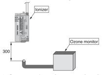
Fig. 2: Ozone condensation measuring circuit
