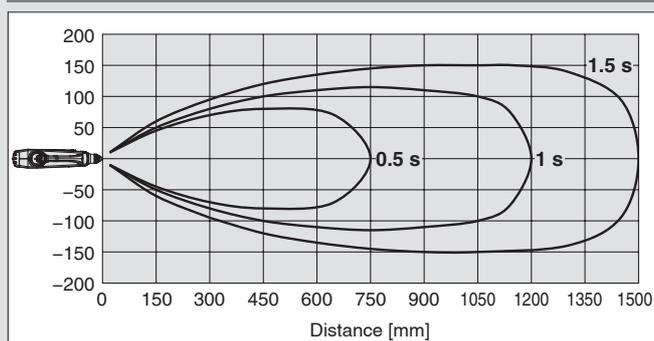
\* Static neutralisation characteristics are based on data using a charged plate (dimensions: 150 mm x 150 mm, capacitance: 20 pF) as defined in the U.S. ANSI standards (ANSI/ESD STM3.1-2015). Use this data only as a guideline for model selection because the values vary depending on the material and/or size of the subject.
