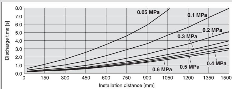
\* Static neutralisation characteristics are based on data using a charged plate (dimensions: 150 mm x 150 mm, capacitance: 20 pF) as defined in the U.S. ANSI standards (ANSI/ESD STM3.1-2015). Use this data only as a guideline for model selection because the values vary depending on the material and/or size of the subject.
