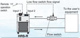
Power for flow switches (24 VDC) can be supplied by the thermo-chiller.
