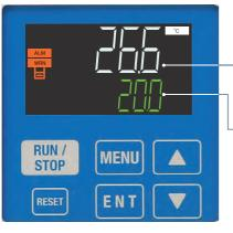
Current value (displayed in white): Discharge temperature, pressure, flow rate, etc.
