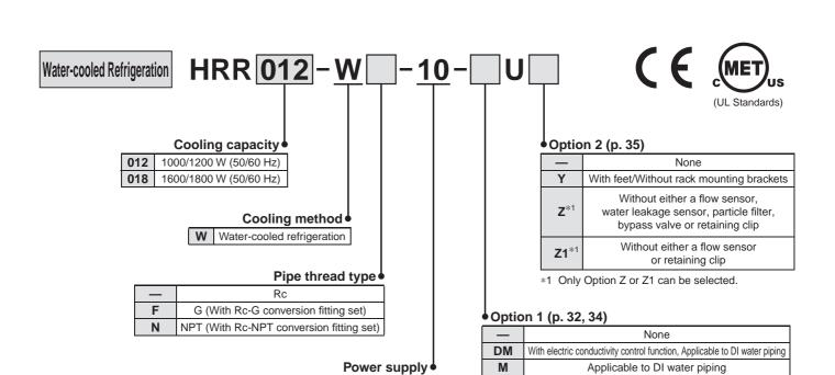
Single-phase 100 VAC (50/60 Hz) Single-phase 115 VAC (60 Hz) High-pressure pump mounted
