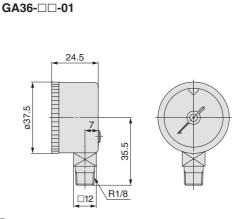
Note 2) Not applicable to water as fluid because its stub is made from aluminum die-casted. Water may cause corrosion and block the air passage.
