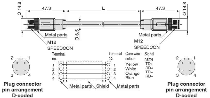
EX9-AC 005 EN-PAPA (With angled connector on both sides (Plug/Plug))
