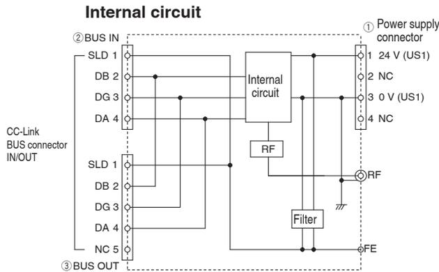
\* The metal housing part of the RF (SMA coaxial connector) is connected to 0 V (US1).
