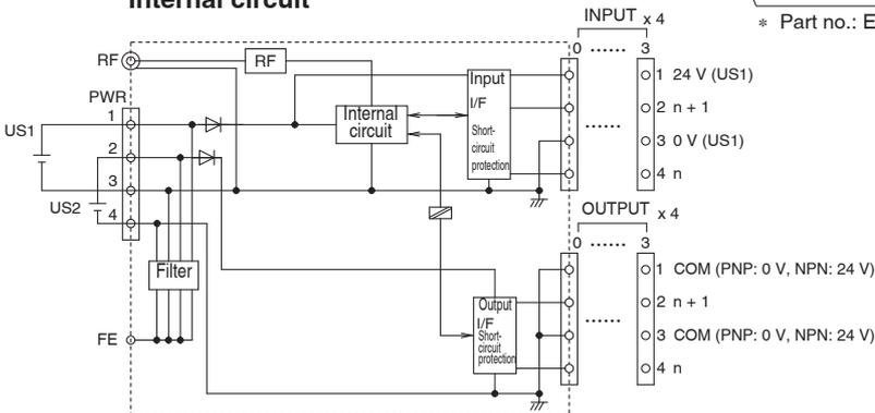
\* The metal housing part of the RF (SMA coaxial connector) is connected to 0 V (US1).
