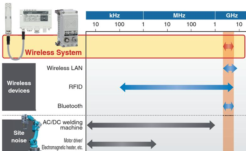
\* ISM (Industrial, Scientific, and Medical) radio bands: Frequency bands allocated for industrial, scientific, and medical applications
