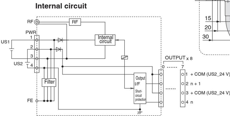
\* The metal housing part of the RF (SMA coaxial connector) is connected to 0 V (US1).
