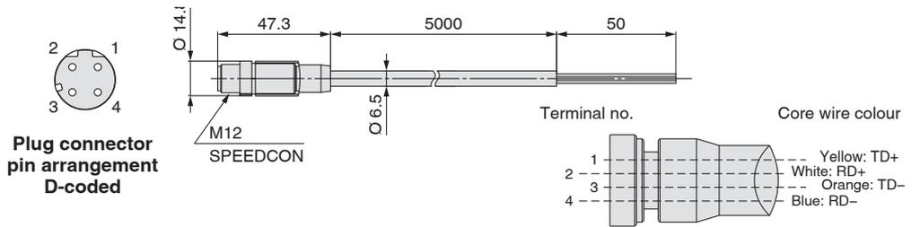
EX9-AC 005 EN-PSPS (With connector on both sides (Plug/Plug))
