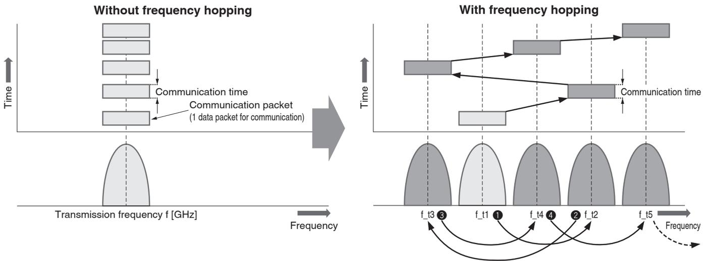
When a source of radio interference is present on a specific frequency, communication is maintained by moving to another frequency.
