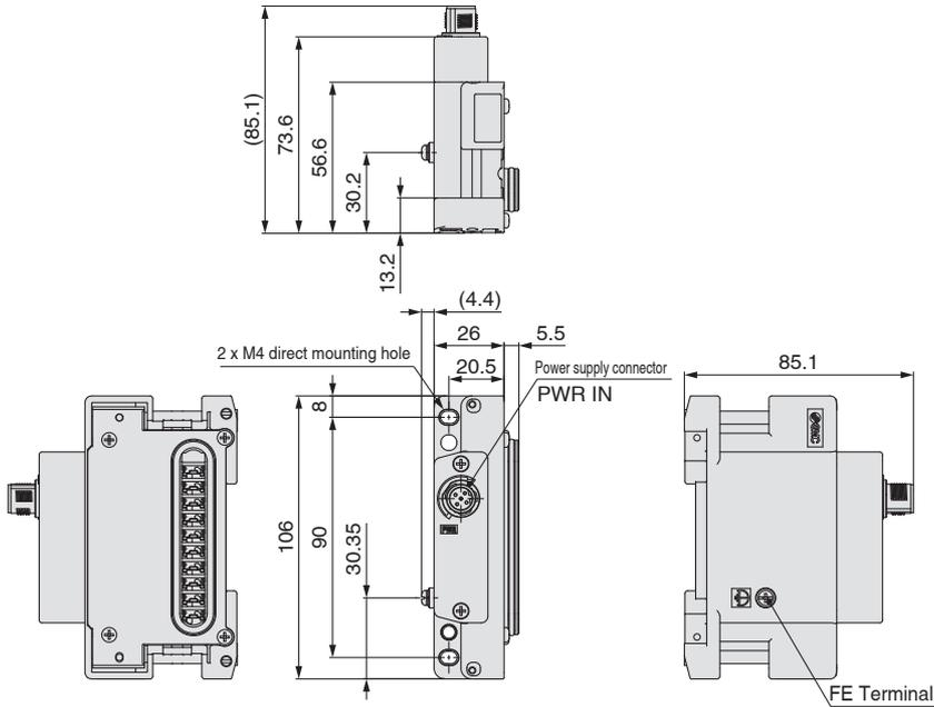
**Power supply connector PWR IN: M12 5-pin plug, B-coded**
