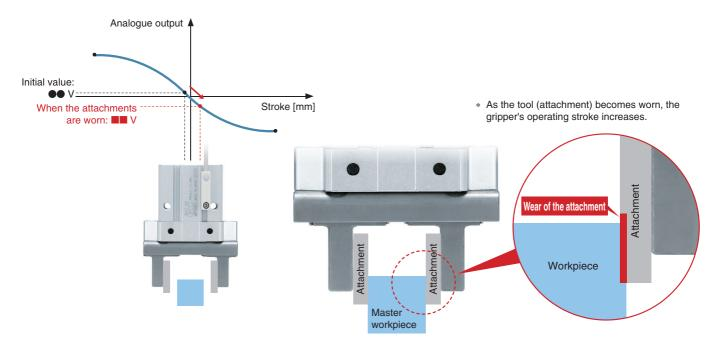
The difference between the measured value and the threshold value can be displayed using the function provided on the display sensor monitor. (Example) When the value at which the master workpiece is gripped is set as the threshold value, the difference can be checked each time.
