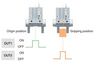
Simple workpiece recognition
