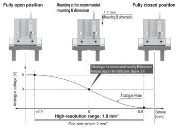
\*1 When mounted on an MHZ2 (Ø 6) air gripper
