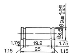
Retaining ring: Type C9 for axis
