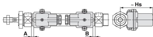
**Auto Switch Proper Mounting Position (Detection at stroke end) and Mounting Height**
