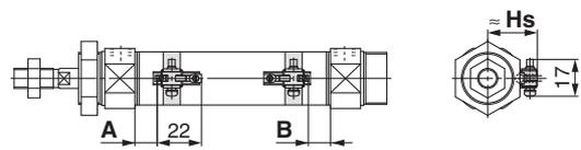
A and B are the dimensions from the end of the head cover/rod cover to the end of the auto switch.
