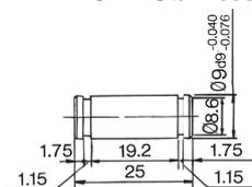
Retaining ring: Type C9 for axis
