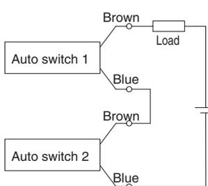
When two auto switches are connected in series, a load may malfunction because the load voltage will decline when in the ON state. The indicator lights will light up when both of the auto switches are in the ON state. Auto switches with a load voltage less than 20 V cannot be used. Please contact SMC if using AND connection for a heat-resistant solid state auto switch or a trimmer switch.
