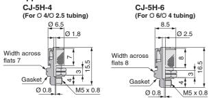
In addition to the above fittings and hose nipples, the below fittings can also be attached to the cylinder. When using the below fittings, be sure to provide a speed controller after adjusting it to 500 mm/s or less.
