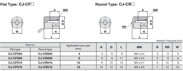
\* Rod end nut is not included when rod end cap is ordered individually. (Please use the rod end nut of the standard cylinder.)
