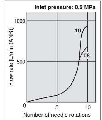
Note) The numbers above the flow-rate characteristic curves in the charts show the tubing diameter as defined by the product number.
