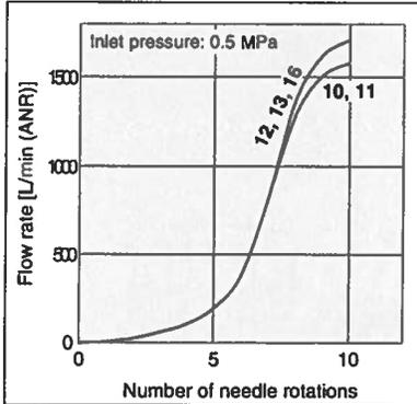
Note) The numbers above the flow-rate characteristic curves in the charts show the tubing diameter as defined by the product number.
