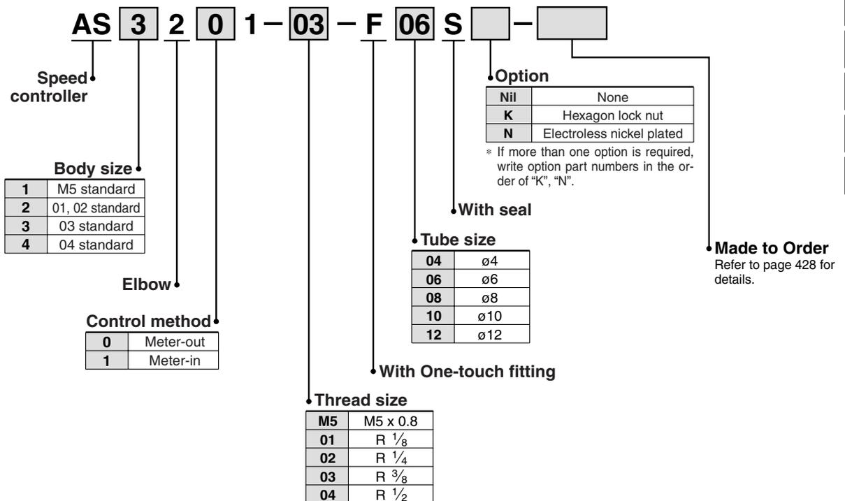
Note 1) M5 size: S (with seal) is not necessary.
