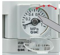
Adjust the indicator using a flat blade screwdriver.
