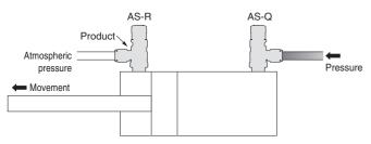
\* Adjust the product when the cylinder operates in the direction of the arrow or completes the operation.
