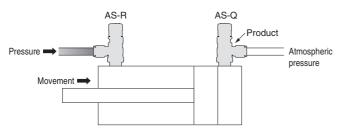
When the product mounted on the rod side is adjusted:
