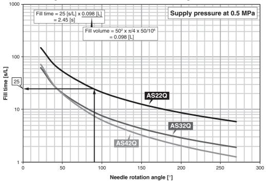
Figure 2. Fill Time Diagram
