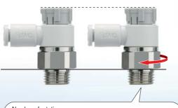
Number of rotations after hand-tightening 1/6 of a rotation or less
