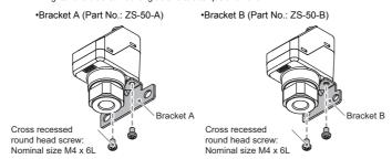
O **Mounting with orifice**\*: Tighten the orifice to a torque of 1.5±0.1 N•m.
