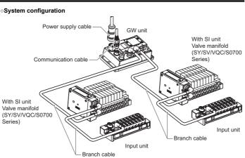
The EX500 range of units can be connected to open fieldbus to realize the reduction of input or output device wiring and the distributed control system One branch of manifold valves/input unit can be connected to 32 outputs/32 inputs Up to 4 branches can be connected (total 128 outputs/128 inputs).
