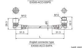
Minimum acceptable cable bending radius: 40 mm (fixed)
