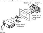
•Mount the bracket using the mounting screws supplied.
