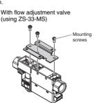
•Install the product (with bracket) using the M3 screws (4 pcs.). Bracket thickness is approximately 1.2 mm.
