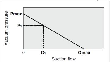
Flow rate characteristics are expressed in ejector vacuum pressure and suction flow. If suction flow changes, the vacuum pressure will also be changed. Normally this relationship is expressed in ejector standard operating pressure use. In the graph, Pmax is maximum vacuum pressure and Qmax is maximum suction flow. The values are specified according to catalog use. Changes in vacuum pressure are expressed in the below order.
