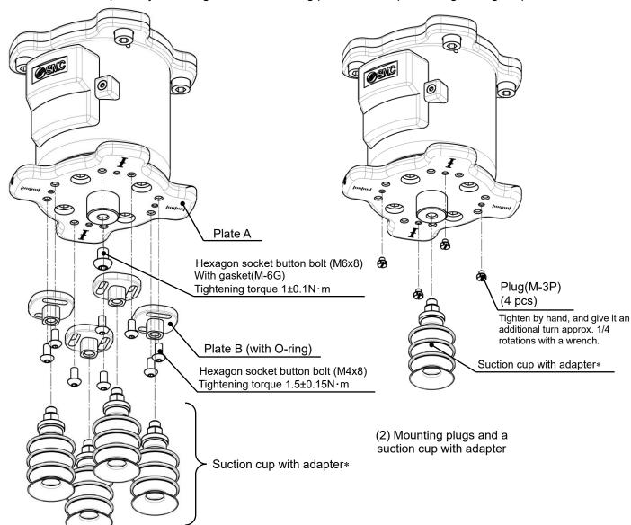
(1) Disassemble the suction cups with adapter
