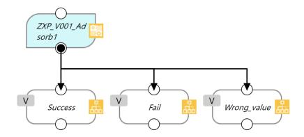
Success: Adsorbs in vacuum and move to the next operation without checking the vacuum pressure level when Adsorb\_and\_ CheckVacuumLevel is set to false.
