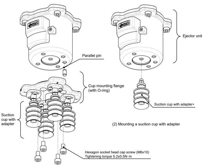
(1) Disassemble the cup mounting flange
