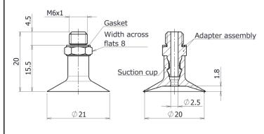
Model: ZPG16J\*-7A-X2 (Suction cup form: Multistage bellows type 2.5-Stage)
