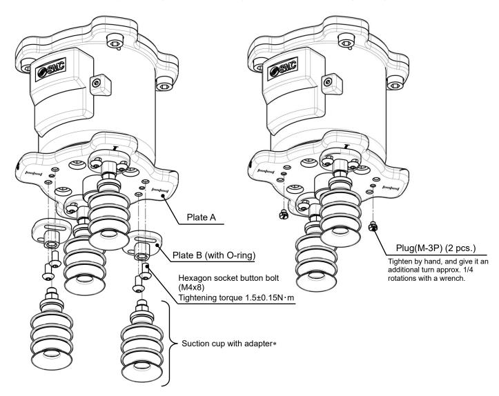
(1) Disassemble the suction cups with adapter
