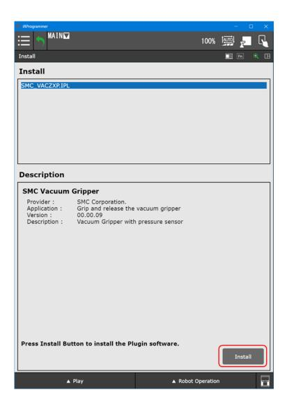
(4) Tap "OK" and install the "SMC Vacuum Gripper" Plugin software.
