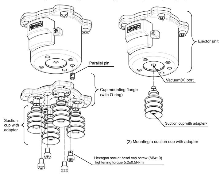
(1) Disassemble the cup mounting flange
