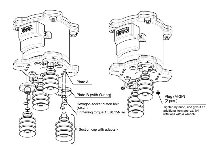
(1) Disassemble the suction cups with adapter
