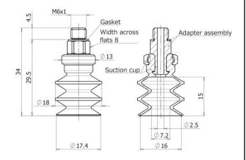
Model: ZPG(B25,B30)J\*-7A-X2 (Suction cup form: Multistage bellows type 3.5-Stage)
