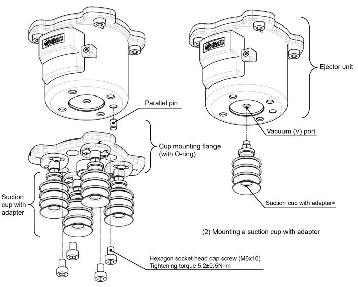
(1) Disassemble the cup mounting flange
