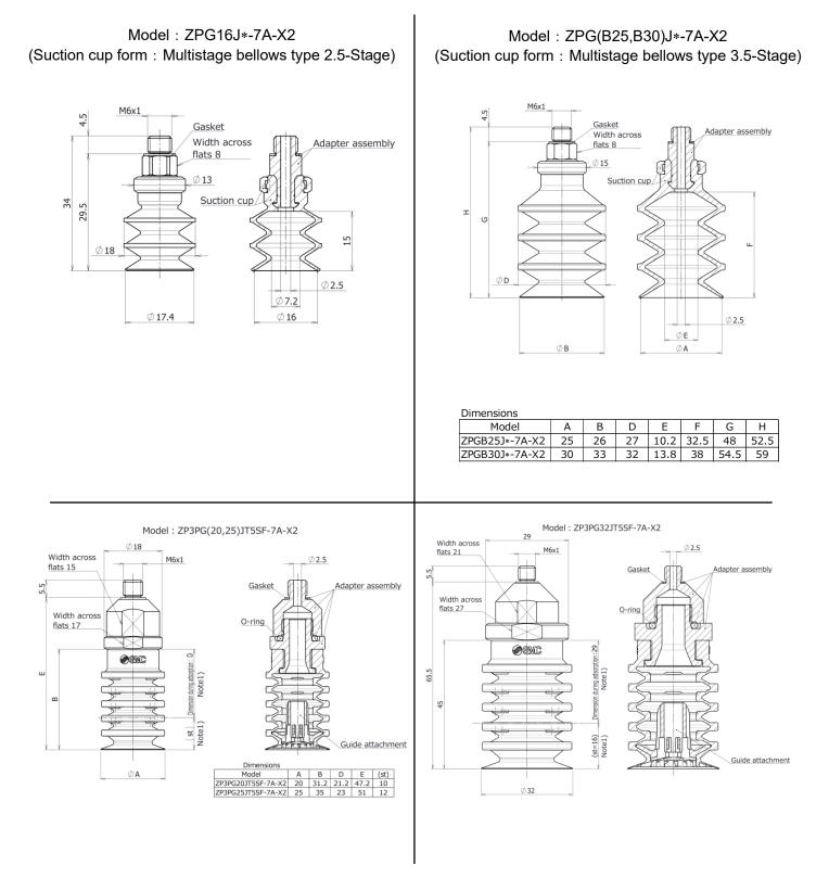
Note1) "D" and (st) indicate the reference value during gripping at vacuum pressure: -85[kPa].
