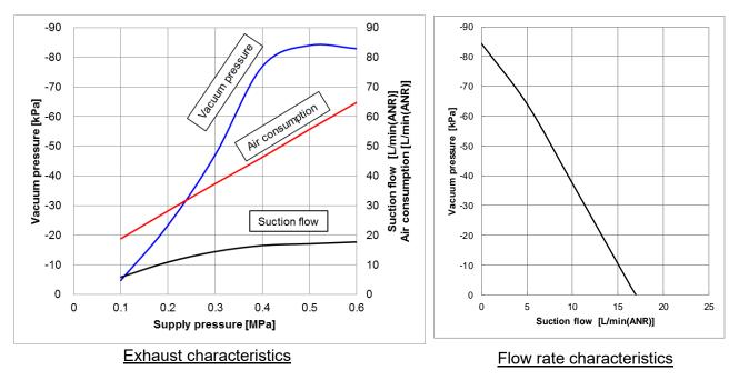
\* The actual suction flow at the point of suction varies depending on the piping conditions to the vacuum port.
