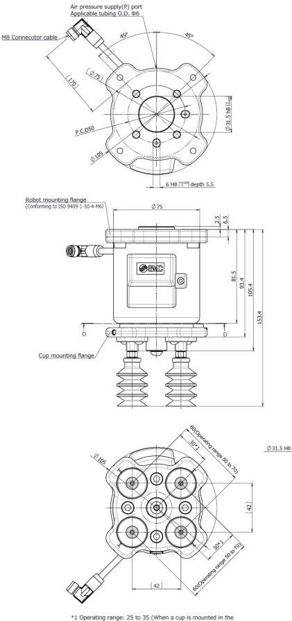
\*1 Operating range: 25 to 35 (When a cup is mounted in the center) As interference between cups may occur depending on the cup diameter, select the cup diameter according to the pitch to be used.
