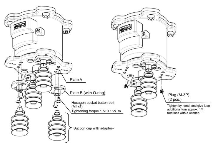
(1) Disassemble the suction cups with adapter
