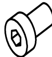
Hexagon socket head bolt (M5 x 25): 2 pc.
