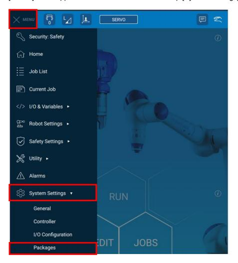
2. Open the [Packages] tab and tap [+ Install] at the top of the screen. A pop-up dialog indicating the packages available for installation will appear. Select "SMC ZXPE5" from the package of and install it
