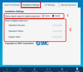
"Status signal output to digital output port"
