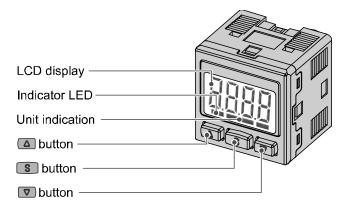
Indicator LED (Green OUT1 and Red OUT2): Displays the switch output condition.
