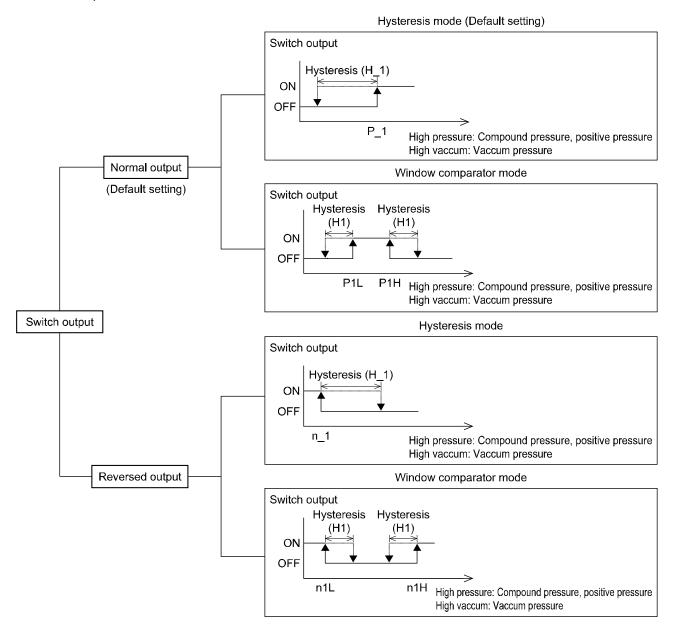
If the set point when the switch output is changed is outside the set pressure range due to switching between normal and reversed output, the hysteresis will automatically be compensated.
