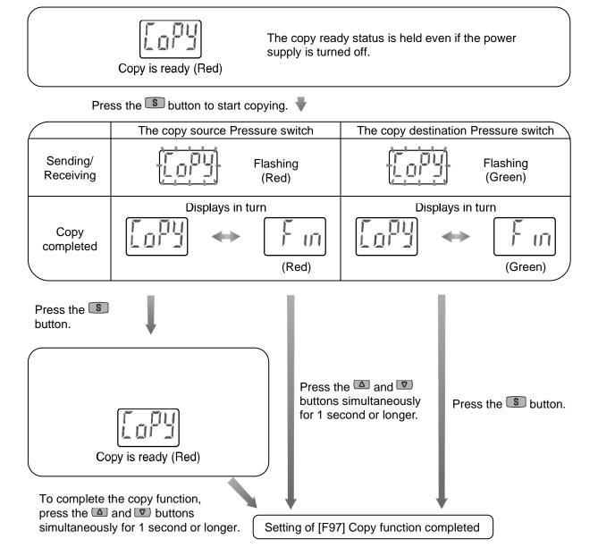
\*: If the copy to the copy destination pressure switch is not completed, it is detected as a copy function sending/receiving error.
