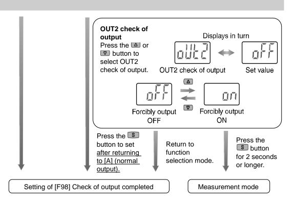
\*: If the subtton is pressed for 2 seconds or longer, the mode is returned to measurement mode regardless of the current mode.
