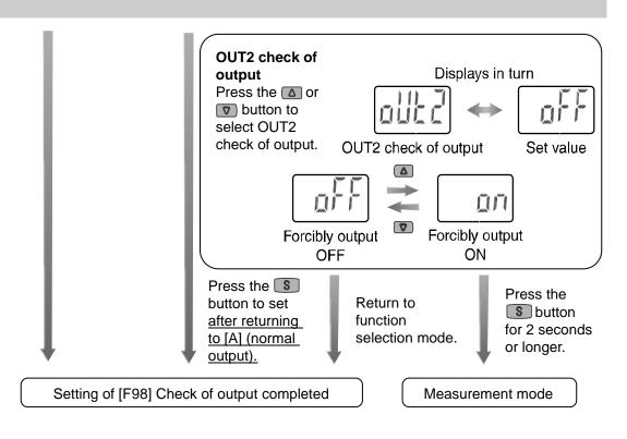
\*: If the S button is pressed for 2 seconds or longer, the mode is returned to measurement mode regardless of the current mode.
