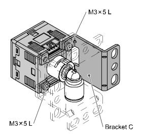
\*: The bracket A/B/C can be mounted in 4 ways.
