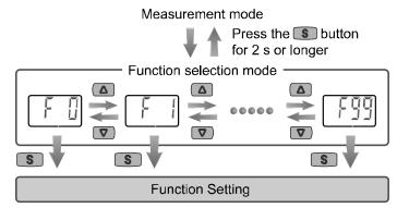
\*: Some functions are not available depending on part number. All functions are displayed with [F  $\Box \Box$ ] followed by the function description. If a function is not available, the function is displayed as [---].
