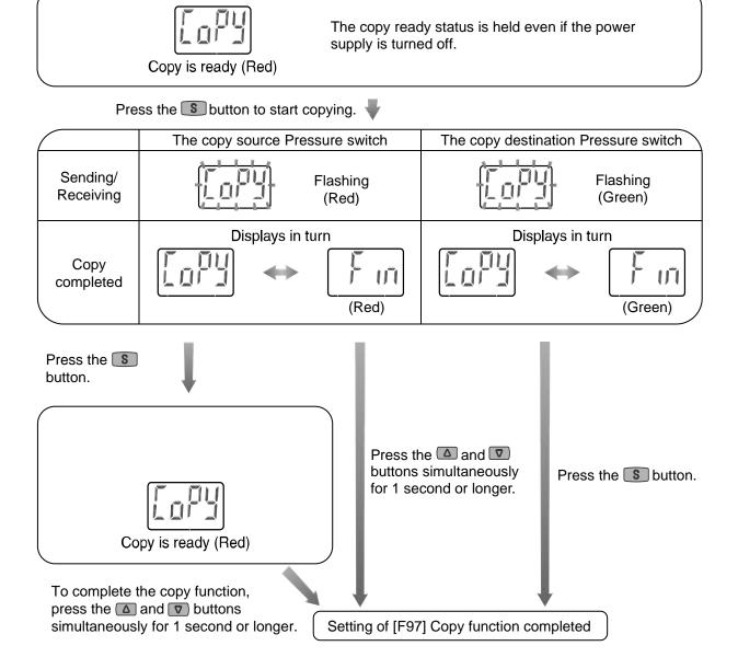
\*: If the copy to the copy destination pressure switch is not completed, it is detected as a copy function sending/receiving error. Press the (a) and (b) buttons simultaneously for 1 second or longer to return to measurement mode. Then, check the wiring and specifications of the switch and retry the copy function.
