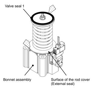
Wipe off any dust from the surfaces of the valve seal 1 and the rod cover.
