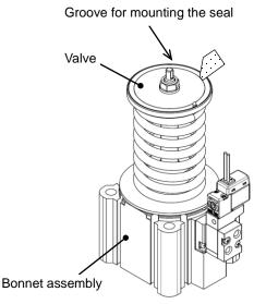
Eliminate any dust within groove for mounting the seal of the valve.
