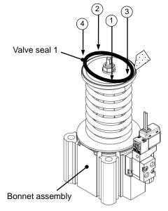
Wipe off any dust on the surface of the valve seal 1, then place the valve seal 1 in the seal mounting groove. Press the seal into the groove in numerical order (press diagonally) to fit the valve seal 1 into the groove. Do not twist the valve seal 1.
