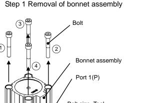
Bolt size, Tool Valve Bolt Hex wrench size size XLFV-16 M4 3 -25 M5 M6 -40 5 -50 **M8** 6 -63 M10 8 -80
