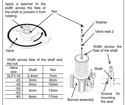
Apply a spanner to the width across the flats of the shaft of the bonnet assembly to hold the shaft, and remove the nut.
