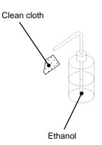
Assemble parts eliminating any dust or debris. Wipe off dust with a clean cloth soaked with ethanol. Blow parts with clean air if necessary. (Ensure there are no fibers or dust.)
