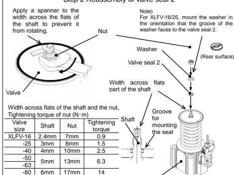
Mount the valve seal 2 and washer.
