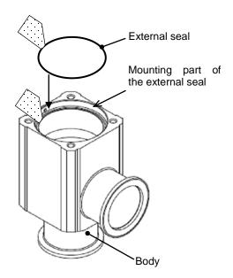
Wipe off any dust from the surface of the external seal and the mounting surface of the external seal on the body, then place the external seal in the mounting position on the body. Step 6 Reassembly of bonnet assembly (No.1)
