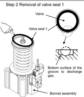
Remove the valve seal 1 from the seal mounting
