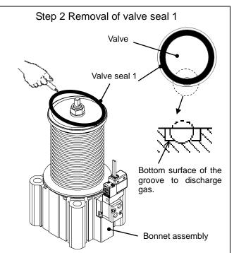
Remove the valve seal 1 from the seal mounting groove.
