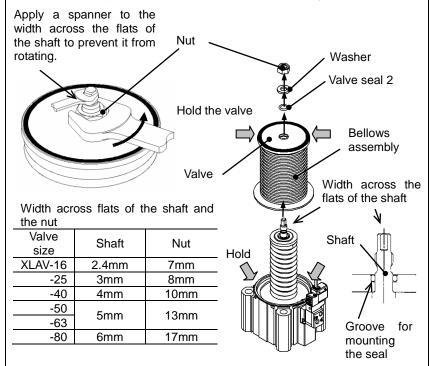
Apply a spanner to the width across the flats of the shaft of the bonnet assembly to hold the shaft, and remove the nut. Be careful not to damage the valve.
