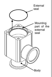
Remove the external seal from the body. (Take care not to damage the surface of the seal mounting groove.)
