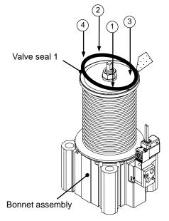
Wipe off any dust on the surface of the valve seal 1, then place the valve seal 1 in the seal mounting groove. Press the seal into the groove in numerical order (press diagonally) to fit the valve seal 1 into the groove. Do not twist the valve seal 1.
