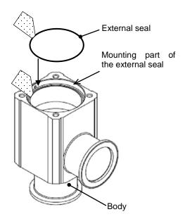
Wipe off any dust from the surface of the external seal and the mounting surface of the external seal on the body, then place the external seal in the mounting position on the body.
