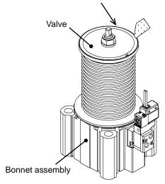
Eliminate any dust within groove for mounting the seal of the valve.
