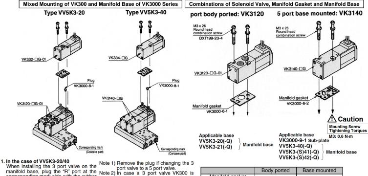
When installing the 3 port valve on the manifold base, plug the "R" port at the corresponding mark side with the rubber Note 2) plug (VK3000-8-1) as shown in the figures on the right.
