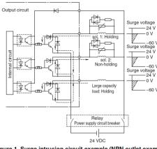
Figure 1. Surge intrusion circuit example (NPN outlet example)
