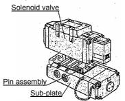
Tightening Torque for Mounting Bolt: 1.1 N·m
